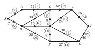
**4 b** To find the maximum flow we will use flow augmentation. Initial network: First, note that the only route with spare capacity from vertex *B* is *BC*. Further inspection shows that we can increase the flow of students by 6 along *SBCDGT*. Updated network:
