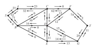
**e** We need to adjust the flow at all arcs to satisfy the flow conservation. The easiest way to do it is to decrease the flow through  $AC_{in}$  to 20 and the flow through FT to 62.
