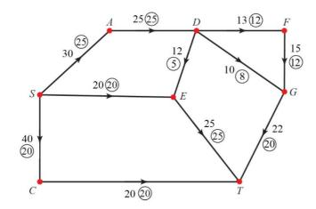
c New value of flow pattern = SA + SE + SC = 20 + 20 + 25 = 65To show that the flow is maximal, first identify all saturated and empty arcs.
