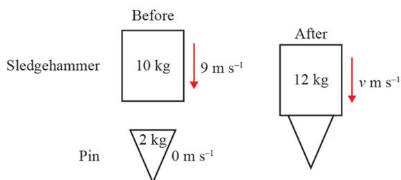
After impact, the sledgehammer and the metal pin move together. You model the sledgehammer and pin as a single particle of mass 12 kg.
