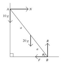
N is the normal reaction at A,R is the normal reaction at B,F is the frictional force at B.
