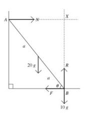
The ladder is on the point of slipping, so  $F = \mu R$
